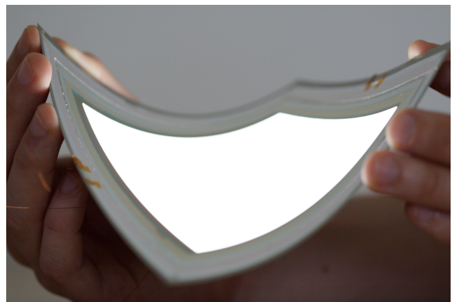
Figure 3 Top emissive OLED (100 cm 2 ) on metal foil thin film encapsulated
